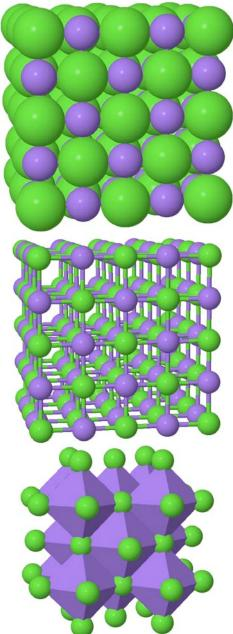
The space-filling model is best for showing relative atom sizes and how the atoms fill space.
