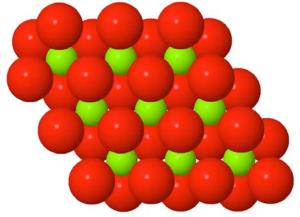
Octahedral spaces between two anion layers in the brucite, Mg3(OH)<sub>6</sub>, structure.
