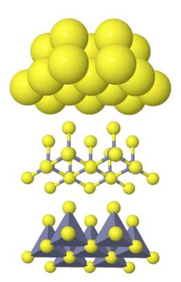
Side view of two anion layers in the zinc blende, ZnS, structure. Which representation best helps you to visualize the structure?
