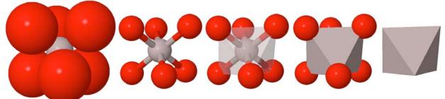
Which of these best represents an octahedral arrangement of atoms? For what purpose? Close packed arrays of oxide ions are the basis of many mineral structures and are important for understanding geochemistry. Geochemists routinely use the representation at the far right.
