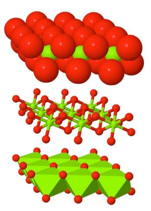
Side view of two anion layers in the brucite, Mg<sub>3</sub>(OH)<sub>6</sub>, structure. Which representation best helps you to visualize the structure?
