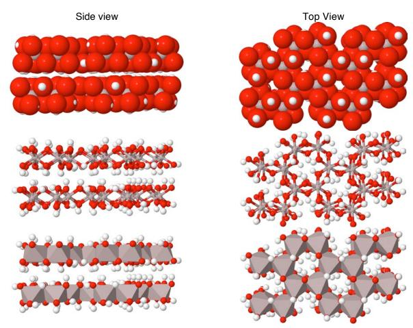
These views also show the hydrogen atoms that are part of  $Al_2(OH)_6$ . In the space-filling representations too large a value has been used for the H<sup>+</sup> ionic radius so that hydrogen can be observed.
