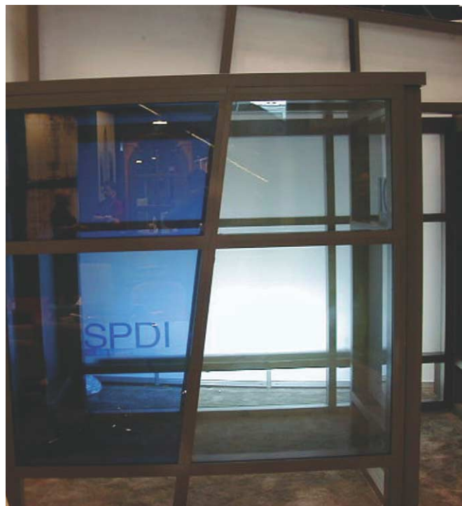
Fig. 5. SPD composite glazing (3 m x 3 m) in four levels of coloration. These windows were shown at the National Glass Association 2002 show in Houston, USA.
