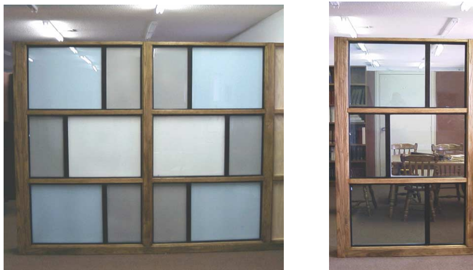
Fig. 7 ThermoSEE thermotropic glazing. The off-state is shown on the left and the heated on-state is shown on the right. (Credit: F. Millett, Pleotint, USA.)
