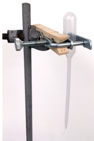
Microtip pipet and Hoffman clamp used for weight titration
