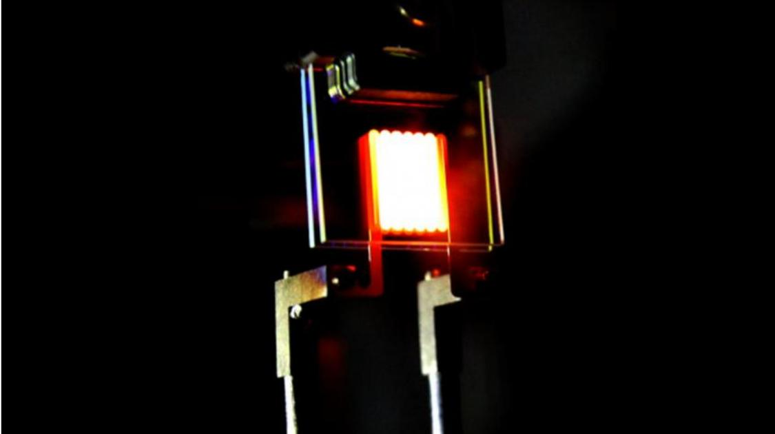
A new type of incandescent light bulb recycles infrared photons converting them to visible light.
