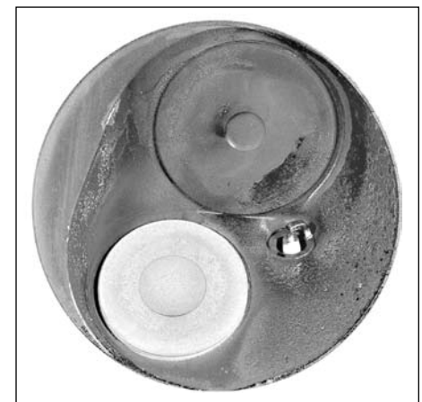
Typical Combustion Chamber Deposits
