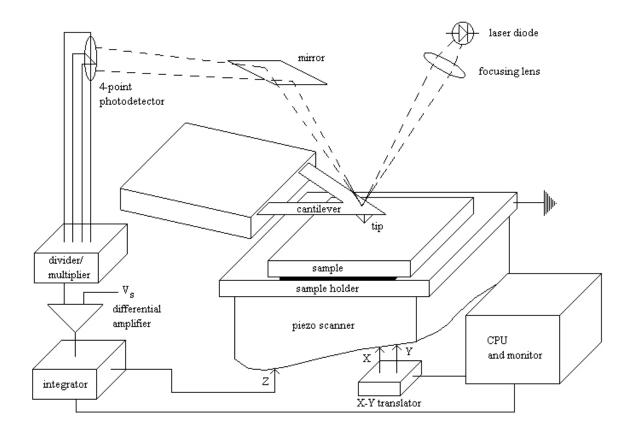
Figure 4. In AFM, small forces are measured between the tip and the sample during scanning. These forces cause vertical movement of the cantilever, which is monitored by a laser beam that is reflected from the top cantilever surface.
