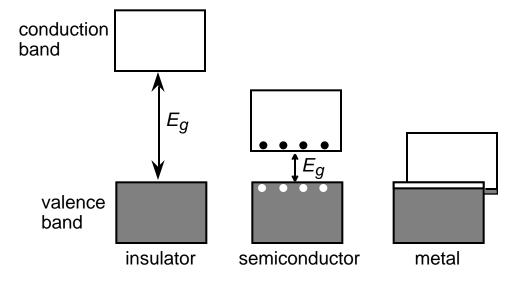
Schematic band-structure diagrams for an insulator, a semiconductor, and a metal. The band gap,  $E_g$ , shown as the double-headed arrow, is the separation between the top of the valence band and the bottom of the conduction band. The size of the band gap energy decreases in passing from an insulator to a semiconductor to a metal. Electron-hole pairs are shown for a semiconductor as filled circles in the conduction band (electrons) and open circles in the valence band.
