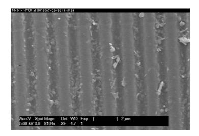
Diffraction grating spacing measured by scanning electron microscopy is approximately 1.8 μm
