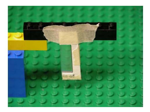
**Note**: Make sure the diffraction grating is aligned so the grooves are parallel to the base and perpendicular to the axis of rotation.
