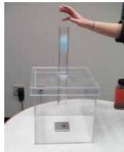
Notice that the weight is in mid-fall in the splatter box. It will hit the paint ball at the bottom of the box, in the center of the aluminum square.
