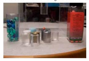
The weights, bath beads, and paints balls used in the splatter box.
