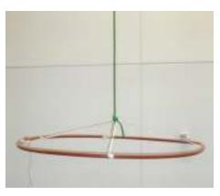
1. Hang the frame with the climbing rope and adjust inner ropes to make the frame level.
