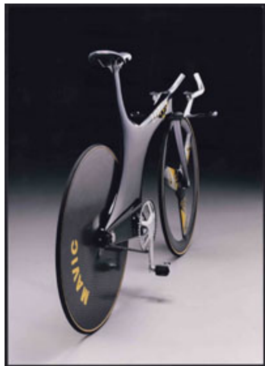
Carbon fiber-reinforced plastics were at the heart of this bike built by Lotus Engineering for the 1992 Barcelona Olympics. It helped Chris Boardman win gold. (Courtesy of Lotus.)
