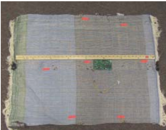
Fig. 3 The cloth sensornet developed at Virginia Tech could help military personnel detect and locate approaching enemy vehicles. (Credit: Zahi Nakad.)
