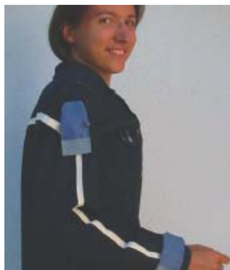
Fig. 5 (a) Researchers at ETH Zürich are using woven fabric with embedded Cu fibers to produce context-aware clothing. (b) Their prototype 'intelligent' jacket uses the conductive fibers to transmit data between different sensors and to measure body movements. (Courtesy of Tünde Kirstein, ETH Zürich)
