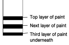
The chemical test solutions are clear (sodium sulfide) or yellow (sodium rhodizonate) liquids. To do the test, the inspector scrapes the painted surface down to the wall surface or substrate. All the layers of paint must be exposed. Then the inspector puts a drop of test solution on the painted surface.
