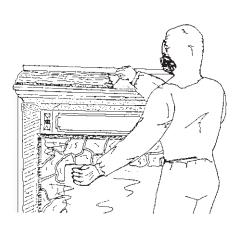
After the paint is removed, carefully clean the surface. Then use a special rinse to neutralize the surface. The rinse balances the acid or base of the stripping chemicals. Check with pH indicators to make sure the neutralizer worked. Repainted surfaces will fail if the caustic paint stripper is not completely removed and the surface is not neutralized. The surface may need to be smoothed and reglued before it is repainted.
