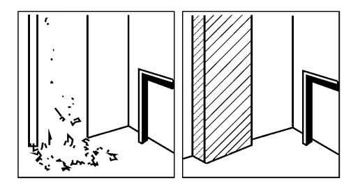
AN ENCLOSURE KEEPS LEAD-BASED PAINT AWAY FROM OCCUPANTS AND THE REST OF THE BUILDING.
