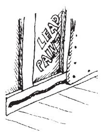
there are building plans, the areas where enclosures cover lead-based paint need to be marked and identified in the plan. This will show workers who work in the building in the future that lead is located there.
