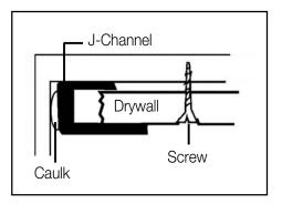
with the finished surface. Screw the drywall in place.
