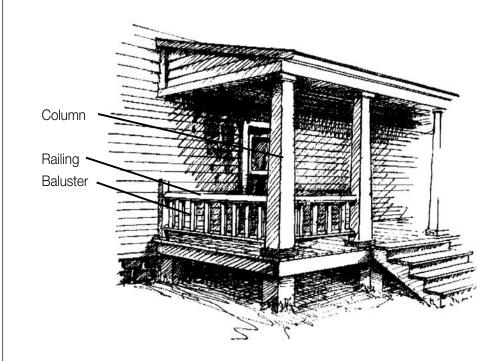
**Porch floors** should be replaced or enclosed. Use treated planks, treated tongue-andgroove, or exterior or marine-grade plywood. Make sure the floor slants down away from the house. The slant allows water to drain properly.
